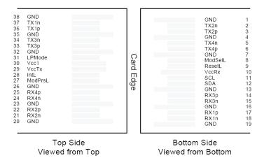
Pin-out of Connector Block on Host Board
